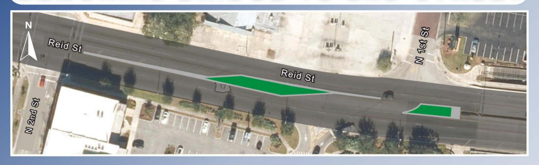
The FDOT and the City of Palatka propose the construction of a median on Reid Street (U.S. 17/State Road 15) from the Memorial Bridge to the intersection of 2nd Street, including a directional opening for eastbound traffic onto North 1st Street.
